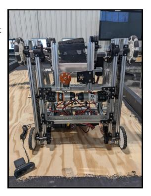
Prior to the season, we had constructed the REV Mecanum Drivetrain Kit, but upon seeing that we would have to cross barriers, we knew our current drive train wouldn't cut it with it's little ground clearance and ability to stick to surfaces. Lucky for us, however, the drivetrain we had was very similar to the REV FTC Starter bot, making it easy to convert it accordingly. Since then, it hasn't seen much change as our current design works quite well.
