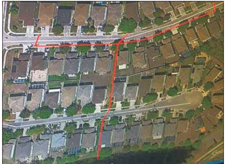
Piping in red along Glenapp Drive (at top) connects to the damaged pipe (at bottom center), which also accepts runoff along Sandgate Ct.
