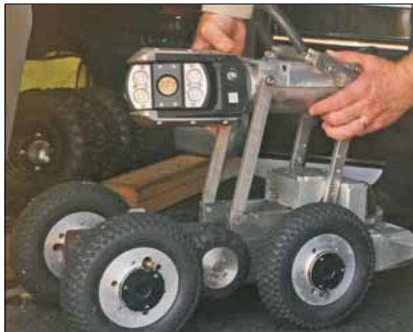
Top photo shows pump at left powering hoses to move water from pond to wetlands in background. At right, vacuum removes water, sand and muck from base of street stormwater drain in front of homes. Photo below shows wheeled camera that rolls through pipes and shows activity, such as water turbulence below bottom.
