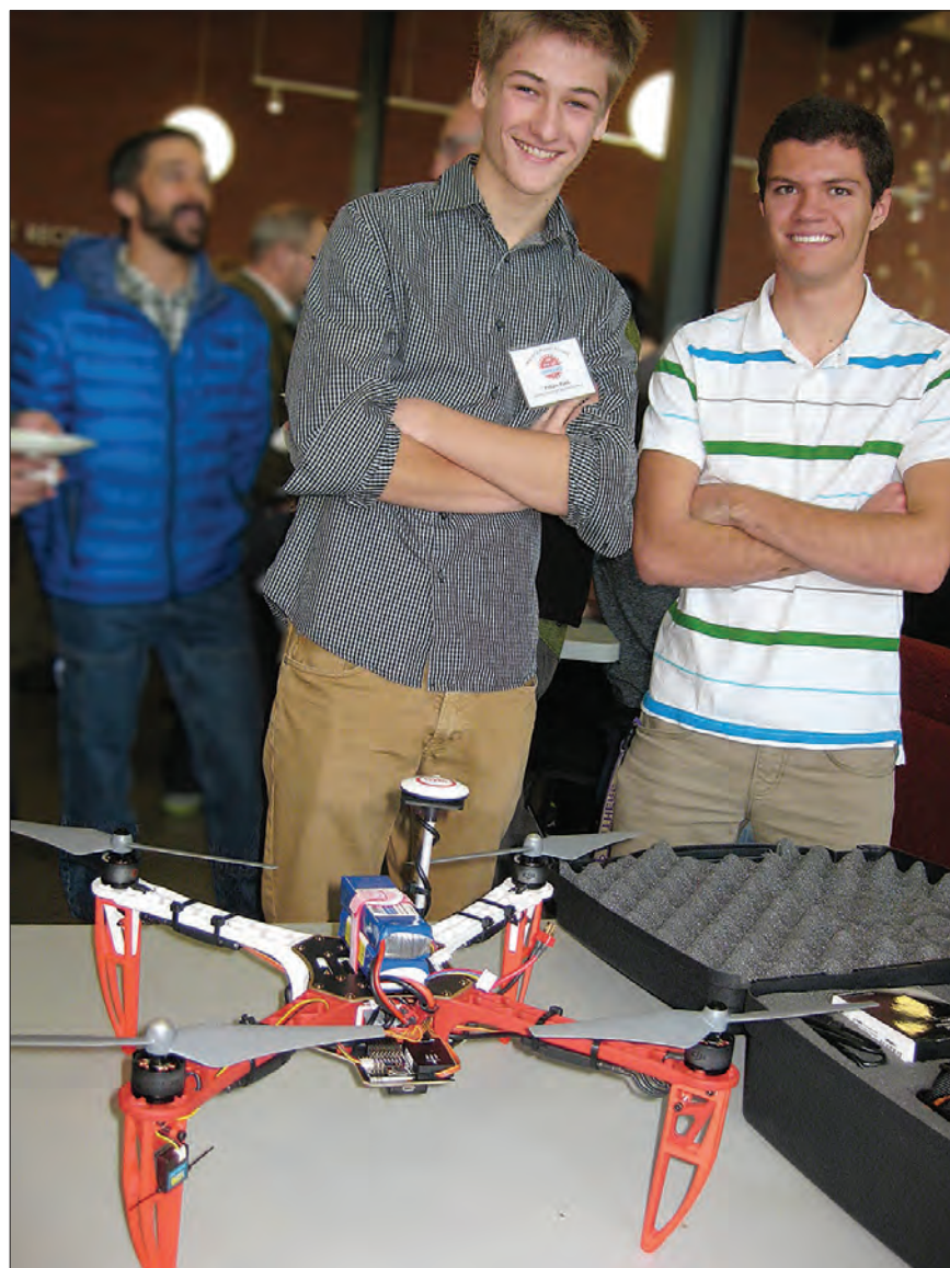
Ethan Toth and Graham Morgan display a Quadcopter at the Mayor’s Maker Forum. Both Toth and Morgan built their own quadcopter, equipped with cameras and GPS. When the copters get out of range they are programmed to fly home.
